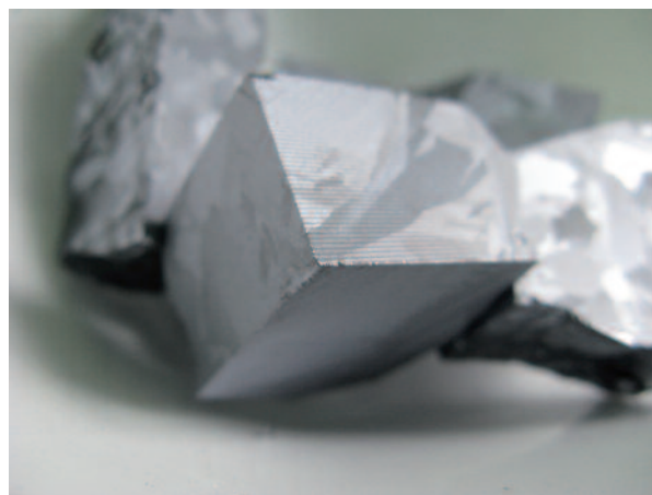
Figure 4: Bricks of multicrystalline silicon base material for the production of solar cells.
